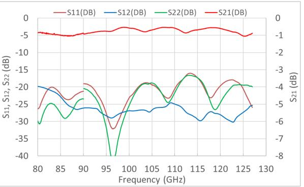
\* WR-9 is a non-standard band. Testing was done in two bands, WR-10 and WR-8. The data was then stitched together at 90 GHz. This accounts for the discontinuity in the reflection data at 90 GHz.
