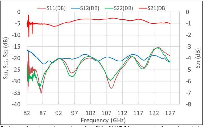
Testing was done at room temperature using a PNA with WR-8 frequency extension modules rated for 90-140 GHz. The ringing below 85 GHz is systemic and not caused by the isolator. Cryogenic tests are coming.
