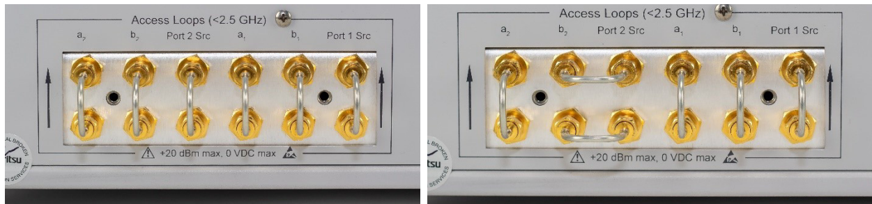
Rear Panel: 'Normal' (left) and 'Reversed' (right) Configurations
