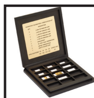
36804B-10M - 10 mil Microstrip Calibration/Verification kit
