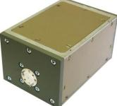
The power oscillator consists of a pulsed IMPATT free-running oscillator, a pulsed IMPATT injection amplifier, two current modulators with chirp compensation and triggering voltage generator. Power output is a waveguide flange, triggering pulse output is a coaxial SMA connector
